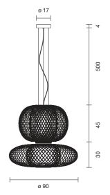
$2\times LED\$  Module ø 70 16,6W 2.700K 1350Lm Light source included - led modules are dimmable with phase-cut dimmers
