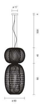
$2\times LED\$  Module ø 70 16,6W 2.700K 1350Lm Light source included - led modules are dimmable with phase-cut dimmers
