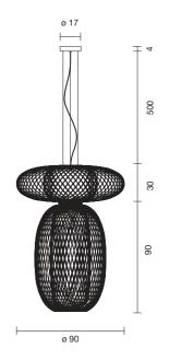
$2\times LED\$  Module ø 70 16,6W 2.700K 1350Lm Light source included - led modules are dimmable with phase-cut dimmers
