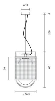
LED Module Ø 46 8,5W 2.700K 680Lm Light source included - led module dimmable with phase-cut dimmers
