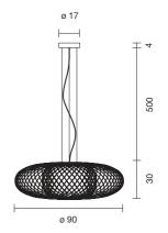
$2 \times \text{LED}$  Module ø 70 16,6W 2.700K 1350Lm Light source included - led modules are dimmable with phase-cut dimmers
