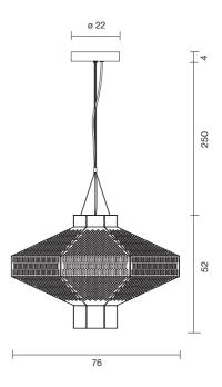
$2\times LED\$  Module 9W 2.700K 1440Lm Light source included - 1-10V dimmable driver included
